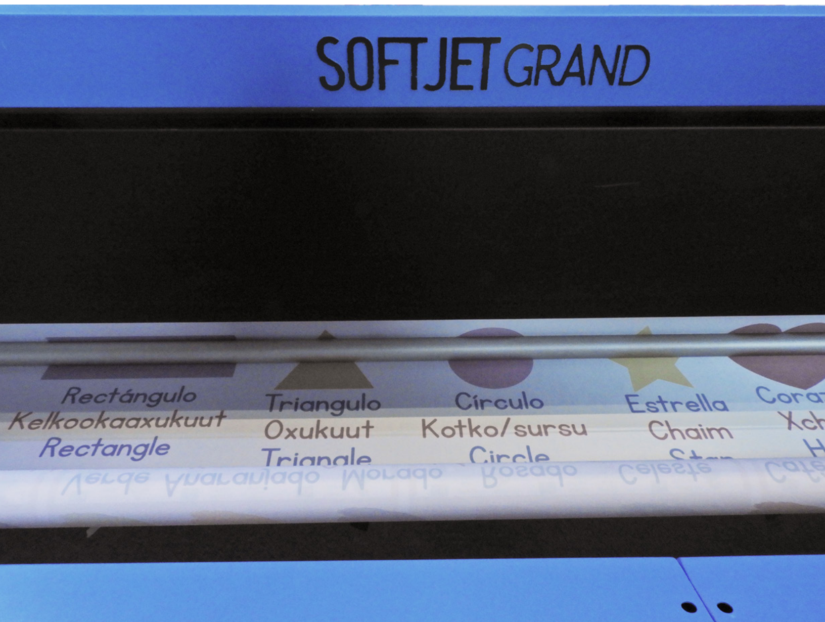
▲ Here is the material on the printer, before it has been heat fixed. The heat fixation will sublimate the ink and brighten the colors dramatically.
