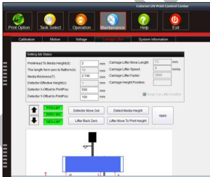
Fig 14: Detecting Head Height
