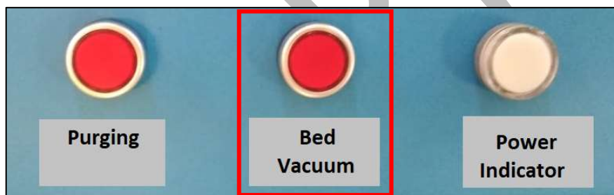
Fig 10: Turning On the Bed Vacuum Button
