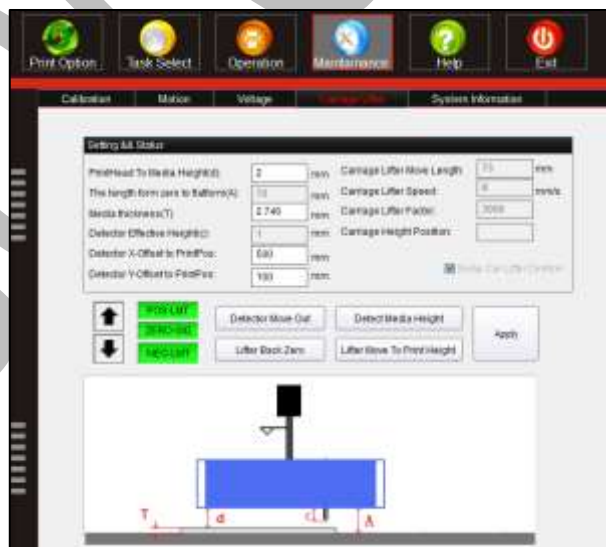
Fig 41: Lifting Up the Carriage
