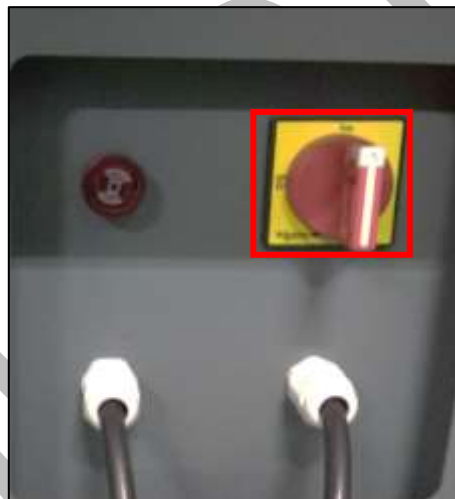
Fig 47: Turn OFF the Main Power Button
