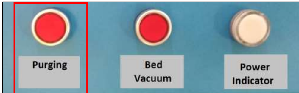
Fig 42: Purging Print Head
