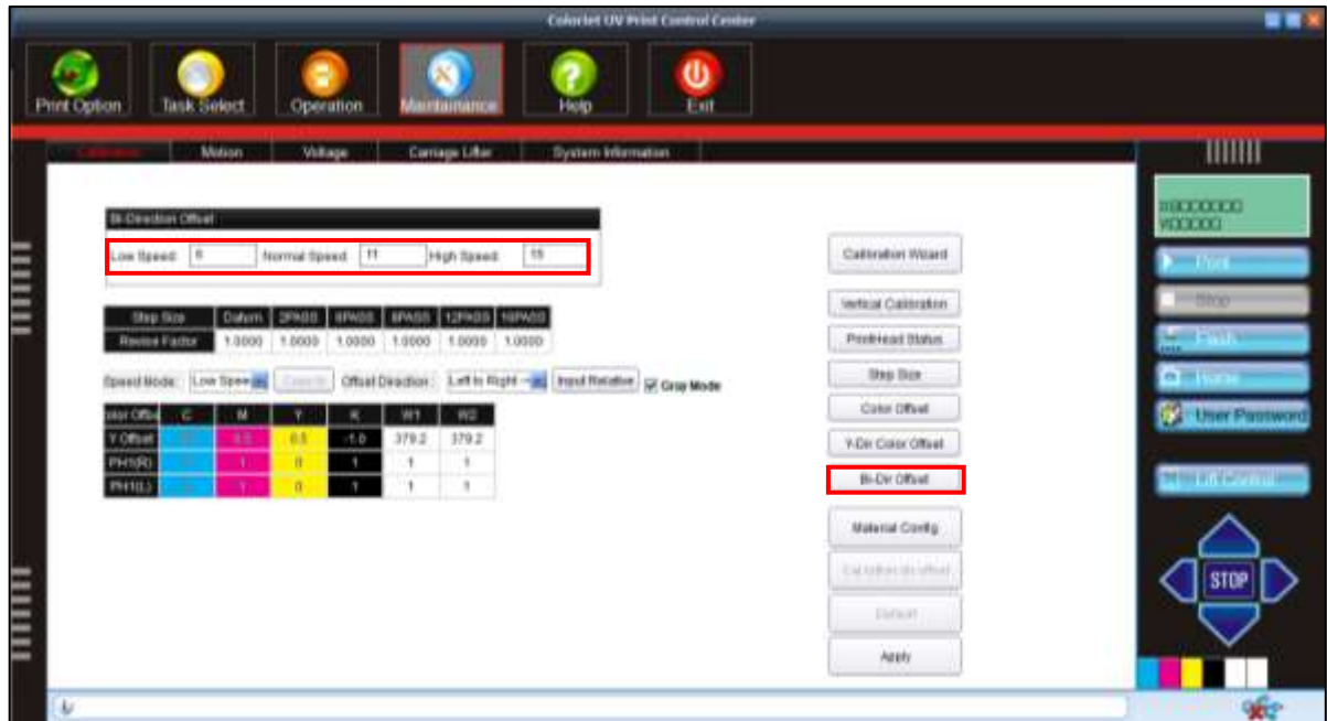
Fig 39: Opening the Calibration Wizard
