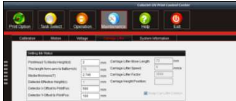
Fig 37: Selecting the Carriage Lifter Tab
