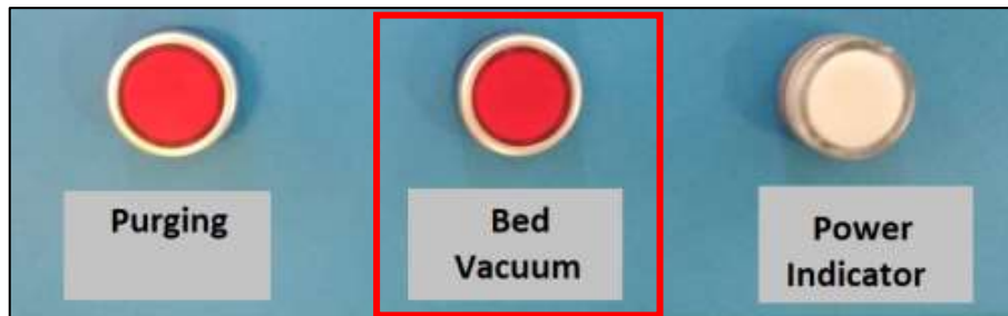
Fig 13: Turning ON the Bed Vacuum Button
