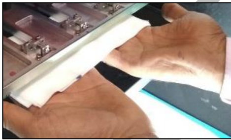
Fig 36: Cleaning the Print Head with a Piece of Cloth
