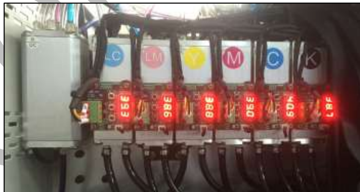
Fig 12: The Sub Ink Tanks with Heaters
