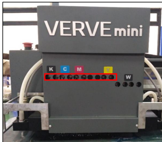
Fig 15: Displaying the Ink Valves
