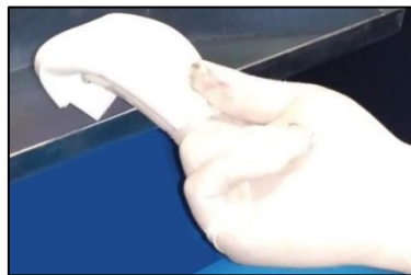
Fig 44: Cleaning the Print Head with a Piece of Cloth
