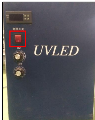
Fig 50: Switch OFF the Chiller Unit
