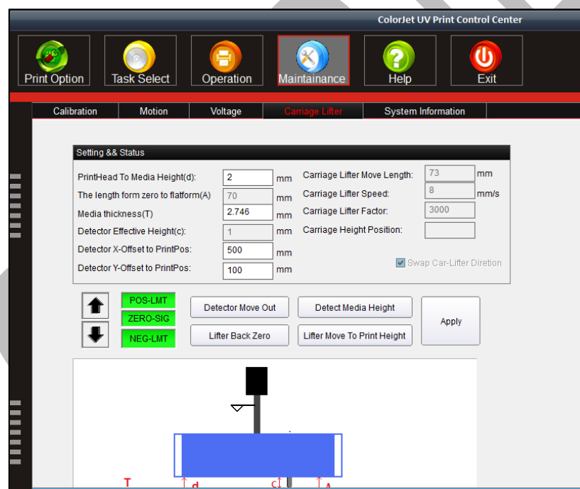
Fig 18: Detecting Head Height
