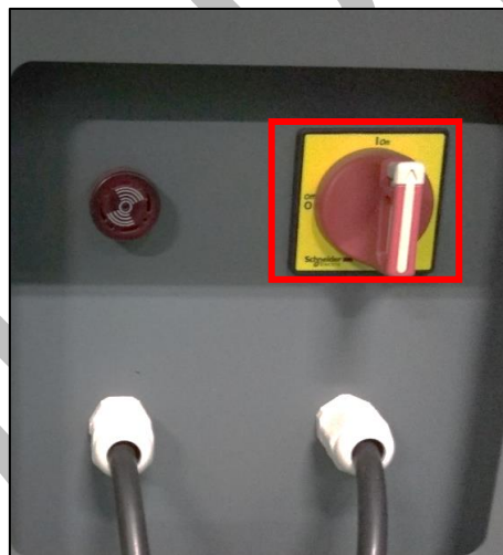
Fig 51: Turn OFF the Main Power Button
