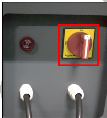
Fig 11: Turning ON the Main Power Switch
