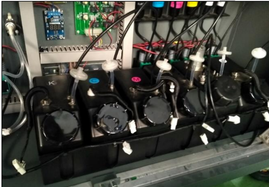
Fig 19: Displaying the Main Ink Tanks and It's Connectors
