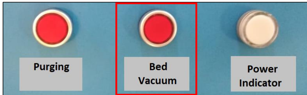
Fig 48: Switch OFF the Bed Vacuum
