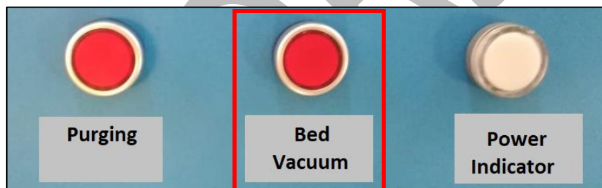
Fig 14: Turning On the Bed Vacuum Button
