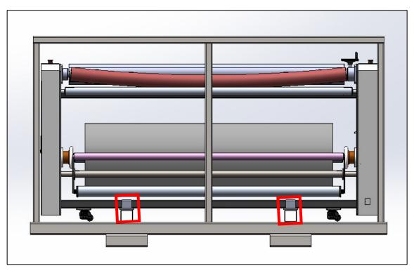
**Step 3:** Insert fork lift arms at the marked shown below by centering and balancing the machine and its parts.
