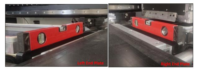
Use the inner corner levellers (fitted with leveler block) to level the machine.
