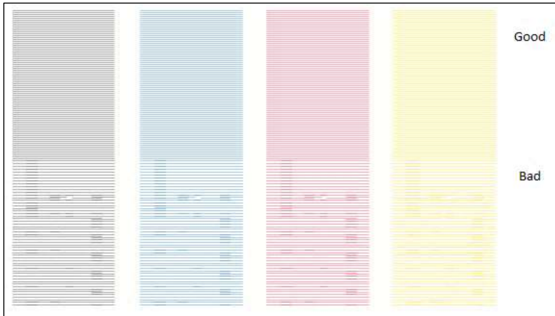
Fig 20: Displaying the Good and Bad Nozzle Test Result
