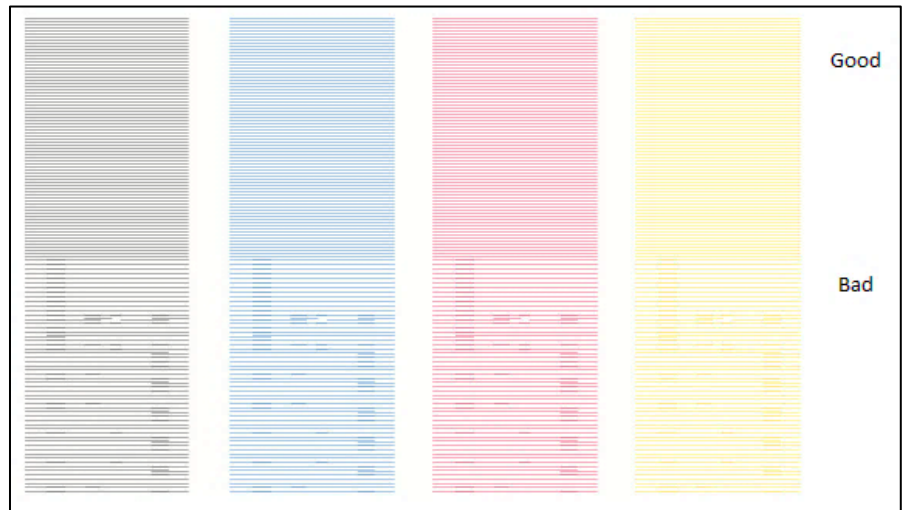
Fig 21: Displaying the Good and Bad Nozzle Test
