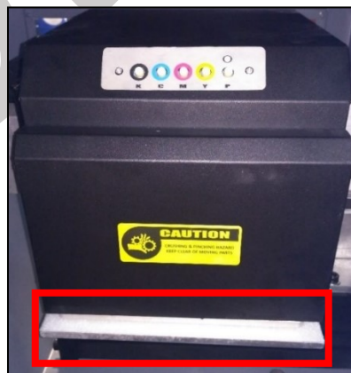
Fig 50: Engaging the Night Plate with Head Plate
