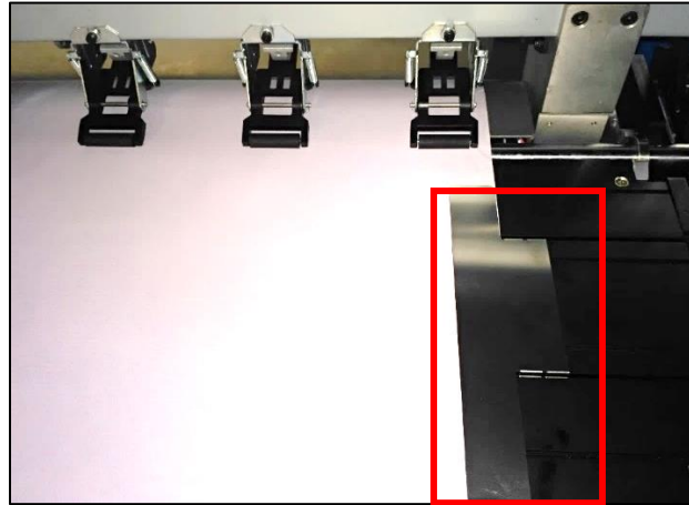
Fig 15: Installing the Media Clamp
