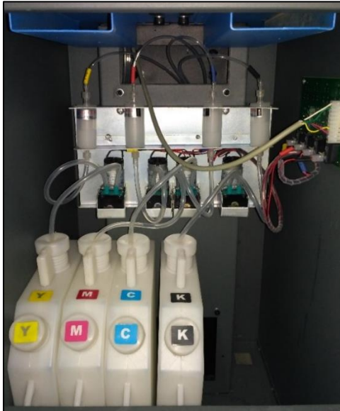
Fig 16: Filling Ink in Main Ink Tank
