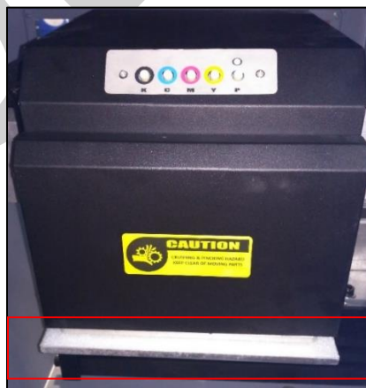
Fig 46: Engaging the Night Plate with Head Plate
