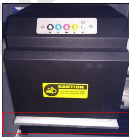
Fig 47: Engaging the Night Plate with Head Plate
