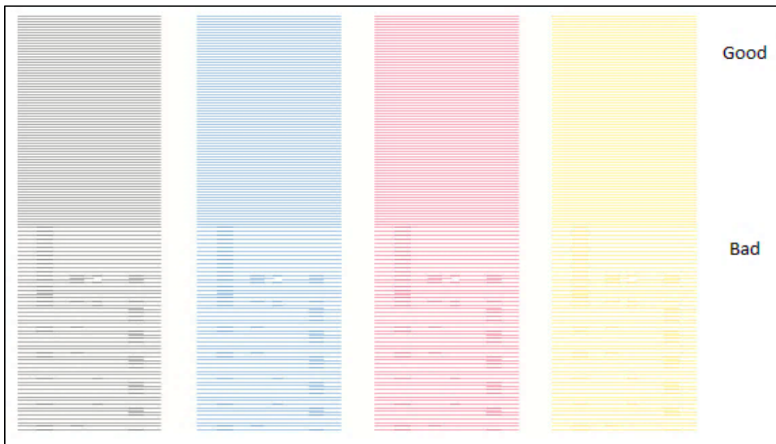
Fig 45: Displaying the Good and Bad Nozzle Test Result
