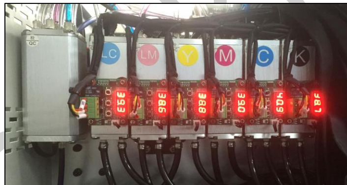
Fig 9: The Sub Ink Tanks with Heaters
